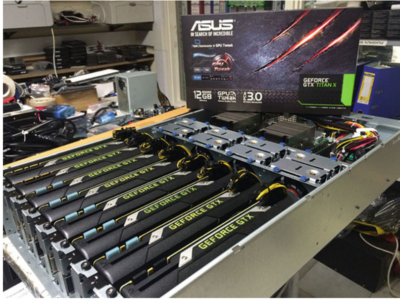
Fig. 3.7 Affordable mini supercomputer for AI: 19" rack server with 8 NVIDIA's Titan Xp GPUs, with 8 \times 3840 = 30,720 parallel cores. Price around 35 K€
