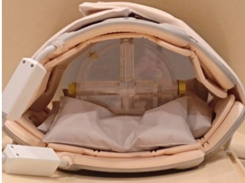
Fig. 16.2 MRI imaging phantom for T1 and T2 calibration (Leeds Test objects, Leeds, UK)
