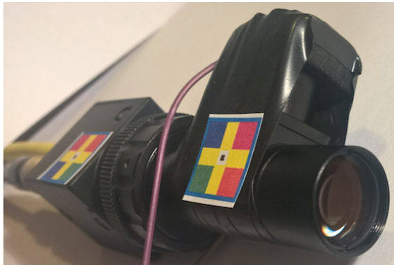
Fig. 5. Dermatological image acquisition camera.
