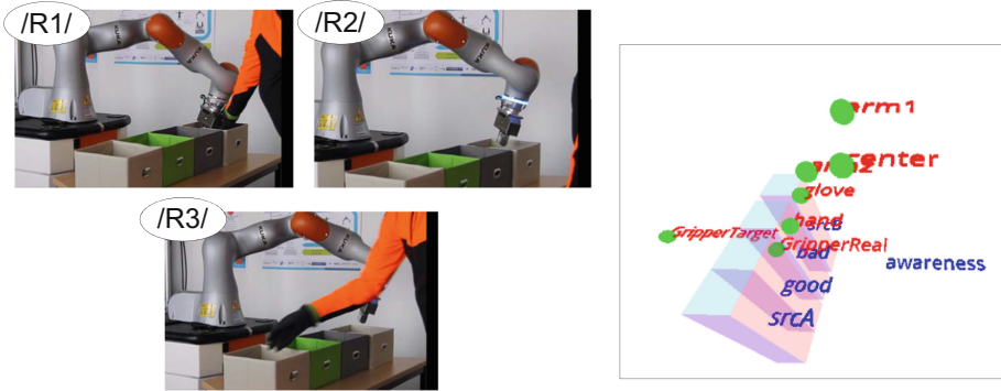
Fig. 5. WEIR collaboration zones for pick-and-place case study. (Color figure online)
