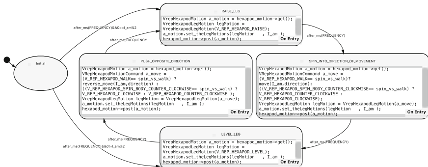
Fig. 7. Executable model for all legs of an n -legged robots as a parameterised LLFSM from which walking gaits and spinning gaits are composed.
