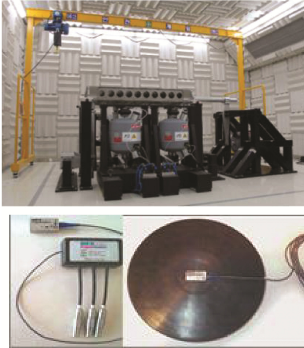
Fig. 2. Multi-axis noiseless BSR exciter simulator ( top ), Vibration Analysis ToolSet, VATS™ ( bottom ).
