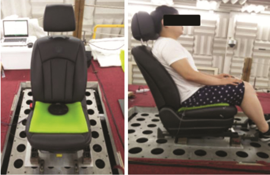
Fig. 3. Experimental setup for measuring vibration experienced by person sitting over balance seat.
