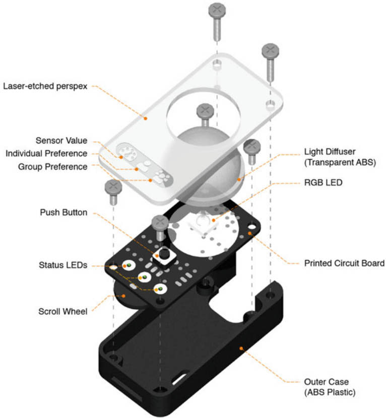
Fig. 3 MiniOrb breakout diagram
