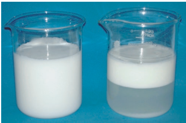
Fig. 18.9 O/W gel emulsions (20 g oil/100 g) using 0.3 g/100 g of high acyl (left) or low acyl (right) gellan gum
