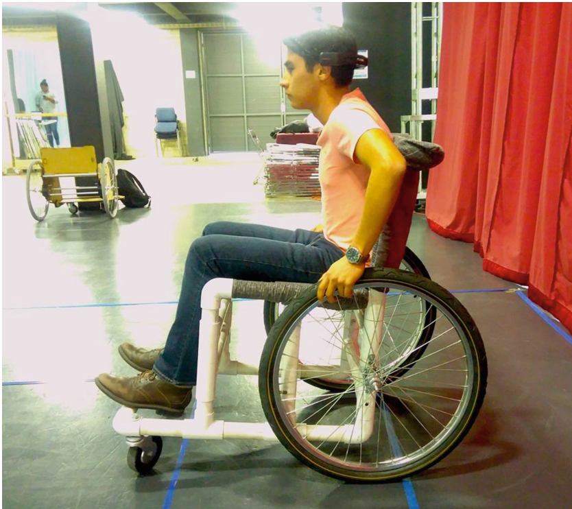
Fig. 8. Participant using the PVC pipes chair during a usability test.
