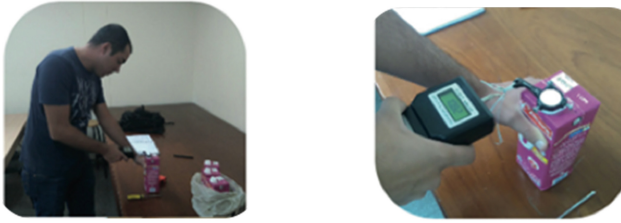
Fig. 5. Required force to open the container
