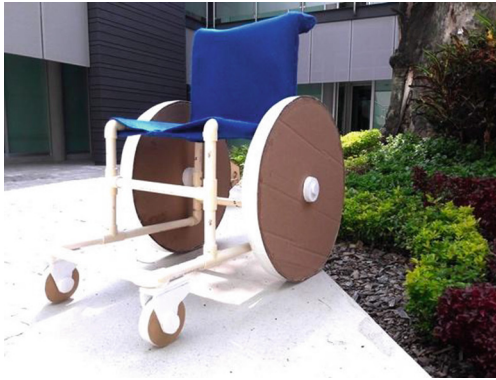
Fig. 5. Scale model of the PVC wheelchair.
