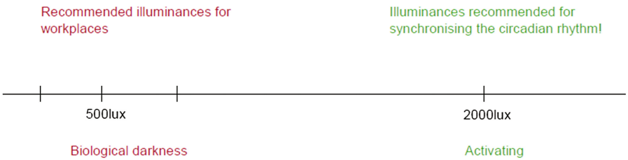
Fig. 3. Illuminance recommended for the optimization of the workplace environment and the synchronization of the circadian rhythm [11].
