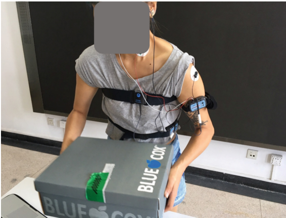
Fig. 3. The placement of the sensors (RSP belt around the breast, PPG attached on the ear, and EDA electrodes on the neck, left and right, and left shoulder).
