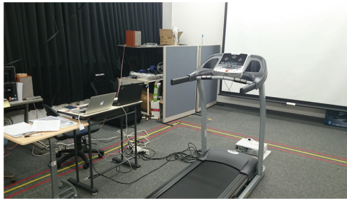
Fig. 2. The treadmill and screen used in the experiment. A projector hung on the ceiling projected the motion picture and a second projector placed on the floor in front of the treadmill displayed the visual targets.
