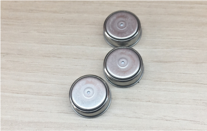
Fig. 2. The temperature and humidity sensors used in this experiment
