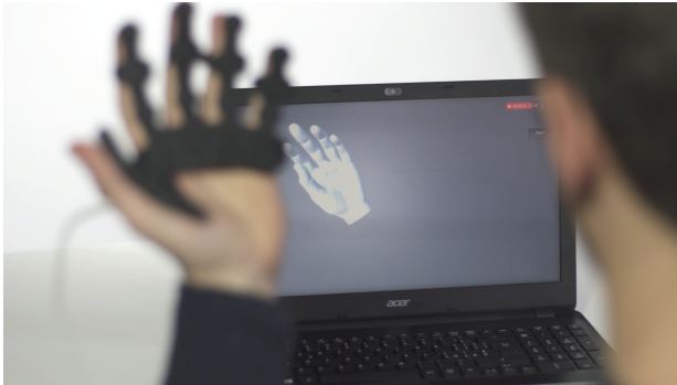
Fig. 1. Acquisition device. Orientation and movement are converted into control signals that enable reproducing the hand in the simulation, in real-time.
