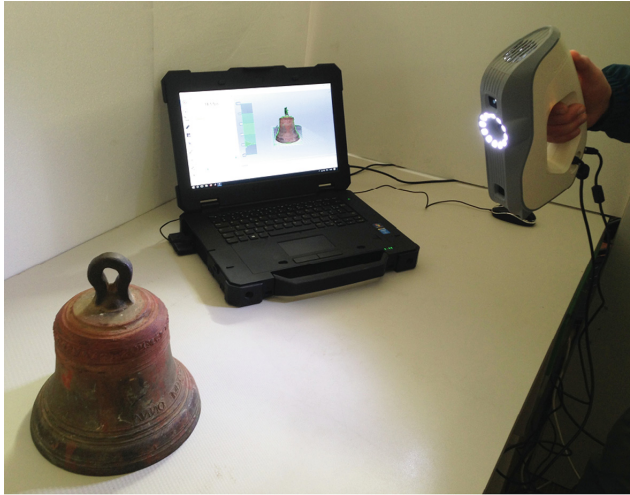
Fig. 2. 3D image scanning of the historical bell with the ARTEC EVA 3D handled scanner
