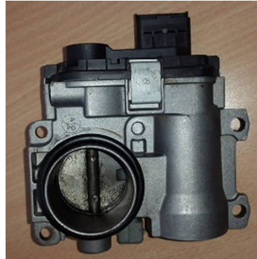
Fig. 3. Electronic Throttle Body (ETB)
