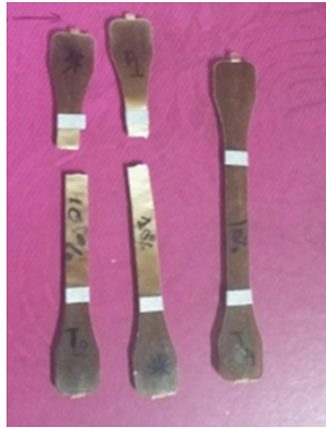
Fig. 6. Specimens before and after rupture.
