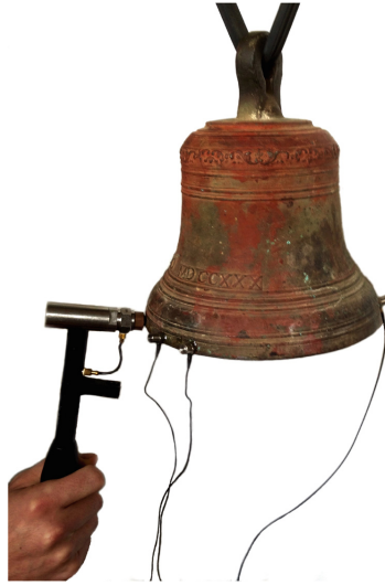
Fig. 6. Experimental test-rig for modal identification. Picture showing the bell suspended, with three accelerometers at the rim and the impact hammer
