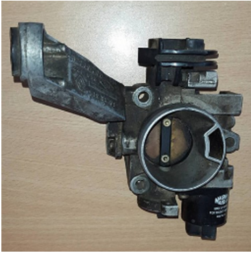
Fig. 2. Throttle Body controlled by cable
