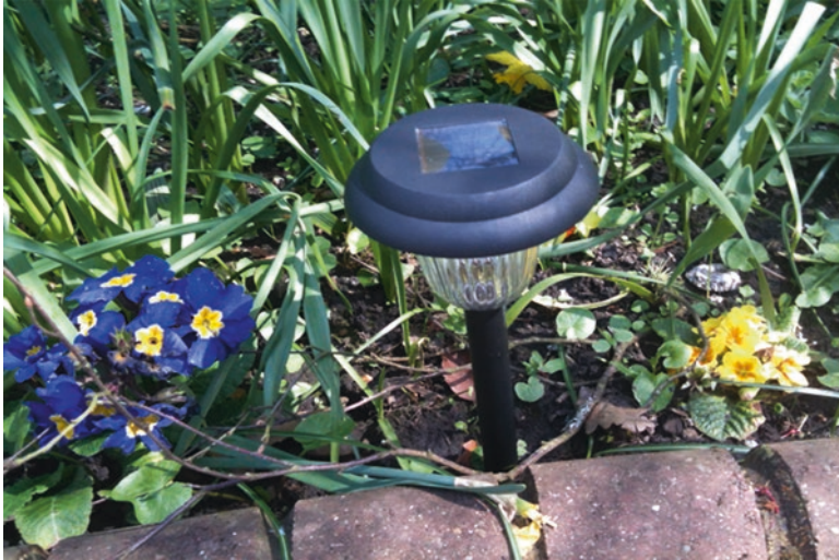
Fig. 36.9 Stand-alone pv usually has a battery to store one night's electrical energy
