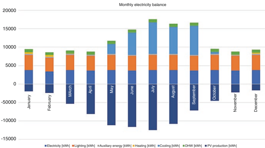
Fig. 33.4 Monthly energy balance in electric consumption and photovoltaic production, considering energy services provided in the building, once renovated
