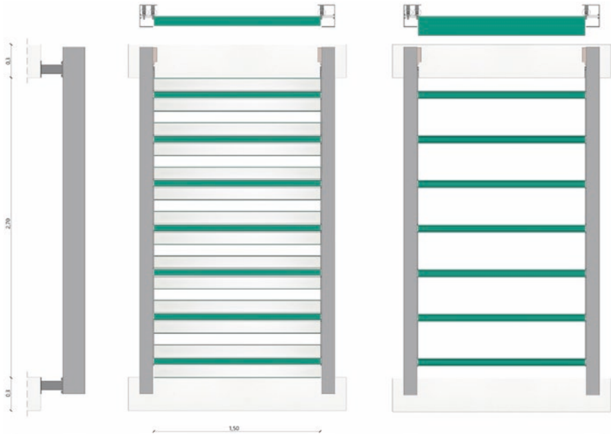
Fig. 28.3 Elevation of the Module in the two positions: open and close
