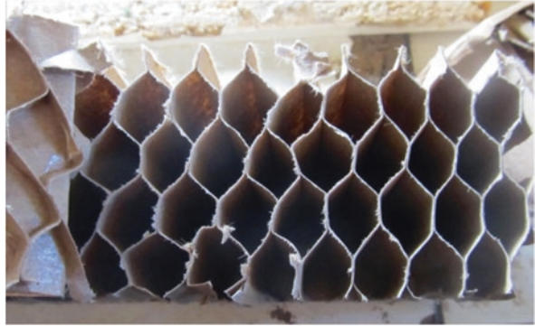
Fig. 39.1 Honeycomb core of the cardboard panel
