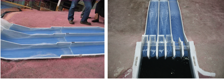
Fig. 1. Water surface profiles along the dam spillway
