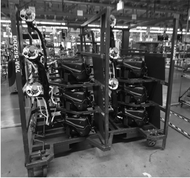
Fig. 1. Sample of the rack from which the tanks are transported and stored at the point of use.
