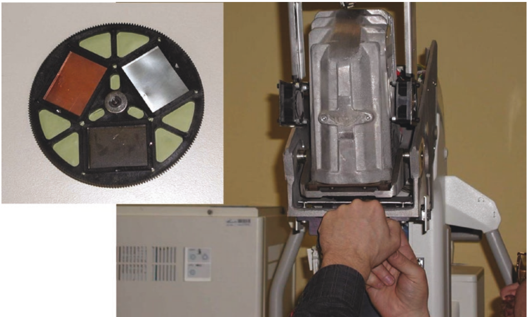
Fig. 4.3 Installation of an additional copper filter for CEDM into the gantry enabling the mammography device to create high-energy images
