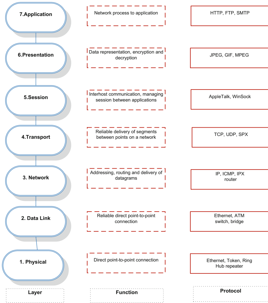
Fig. 2.6 OSI model: layers, function and protocol
