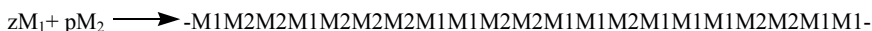
Fig. 4.16 Schematic representation of copolymerization reaction and the corresponding copolymer macromolecule (the reaction is not balanced, and z and p are initial numbers of \text{M}_1 and \text{M}_2 , respectively)
