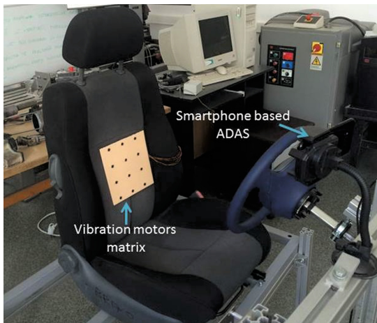
Fig. 2. Vibrotactile motors matrix positioned on the driver's seat and smartphone based ADAS system integrated in a vehicle simulation test bench.
