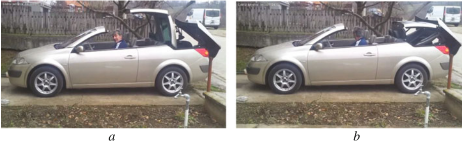
Fig. 1. Pictures of 2-position convertible car mechanism [1]
