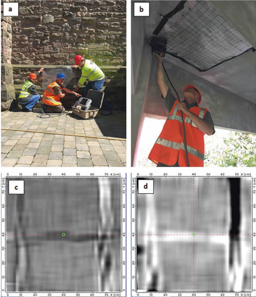
Fig. 4.1 Sideways and upside-down-looking GPR. (a) Example of the use of sideways-looking radar to detect voids in an historic masonry wall (Adapted from Johnston et al. 2018) using 1.2 GHz, 1.6 GHz and 2.3 GHz antennas, courtesy of Mike Langton (Mala Geoscience). (b) Use of upside-down GPR to image a modern concrete bridge, with basalt-fibre rebars using 1.2 GHz and (this image) and 2.3 GHz antennas, results in (a, c and d). (c) Mapped 2.3 GHz output from the survey shown in (b), at 10 cm depth, with basalt-fibre rebars. (d) Mapped 1.2 GHz output from the survey shown in (b), at 15 cm depth, with basalt-fibre rebars (Yeboah et al. 2013). Note the polarity phase change (white/black) with different depths/antennas in (c, d)
