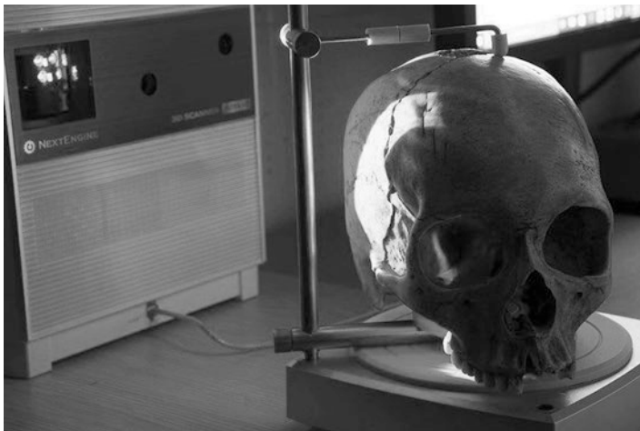
Fig. 8.1 NextEngine tabletop 3D laser scanner in operation, showing skull with cranial trauma being scanned on the turntable
