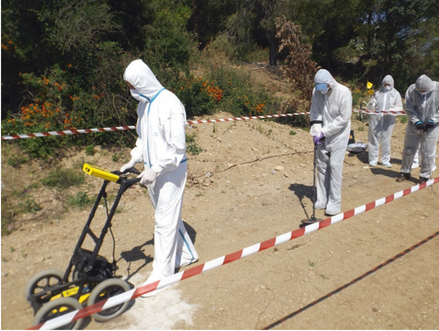
Fig. 3.1 The use of both electromagnetic instruments—GPR and metal detector—in a crime scene
