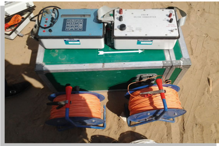
Fig. 5 The used Earth resistivity instruments (ELERIC-T, SYSCAL R2)
