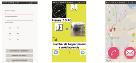
Fig. 1. On the left, menu to save and collect the information; on the center, menu showing the step information and, on the right, map showing the GPS coordinates of the path and the emergency buttons. (Color figure online)
