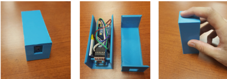
Fig. 1. A tangible with sensor package embedded in the 3D-printed enclosure
