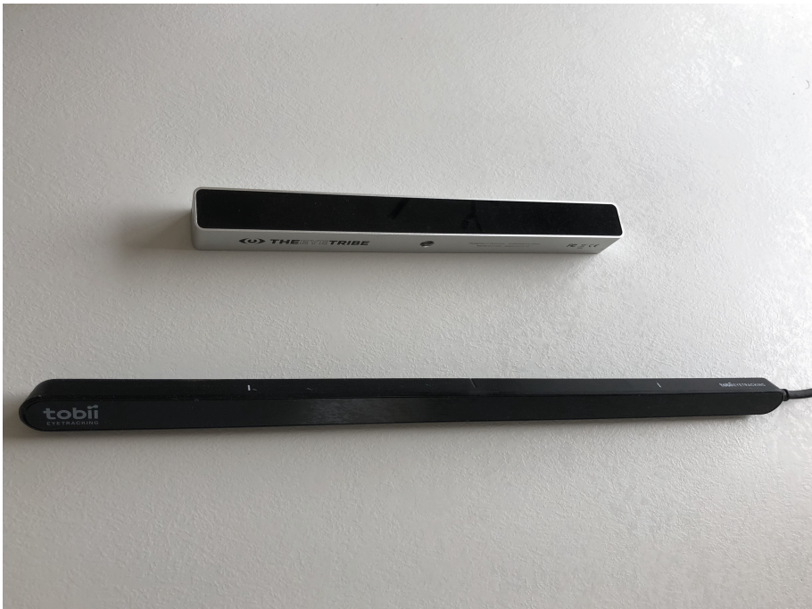
Fig. 1. Two of the eye-trackers which permit to play with GazePlay: the Eye Tribe upper side, the Tobii 4C bottom side
