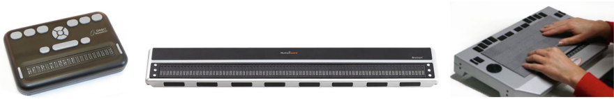
Fig. 3. Typical Braille-Display configurations: left: Orbit 20 ( www.aph.org/orbit-reader-20 ); centre: Brailliant 80 ( www.humanware.com/brailliant ); right: Hyperbraille [21]
