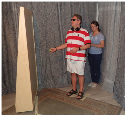
Fig. 1. Localization of obstacles by echolocation in a padded room using a mechanical clicker.
