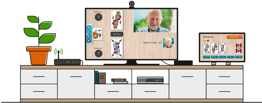
Fig. 2. The BRELOMATE client system consisting of a set-top box connected to a TV for visualisation and a tablet client mainly for control. The screens show the turn-based card game service Schnapsen with the open game table and integrated video-conferencing on the TV and each players individual hands on their tablets.
