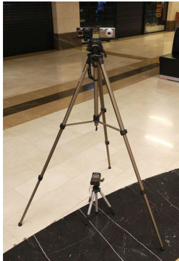
Fig. 3. Stereo rig and the laser rangefinder
