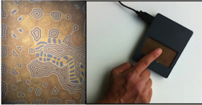
Fig. 1. The painting “Dream of the snake” and the touch stimulation device STIMTAC
