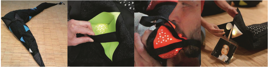
Fig. 1. Parts of Polly World: 1. Banana shaped Interactive object, 2. Bend sensor, 3. Microphone, 4. RFID-reader and music-tune RFID-tagged cover (Michael Jackson).
