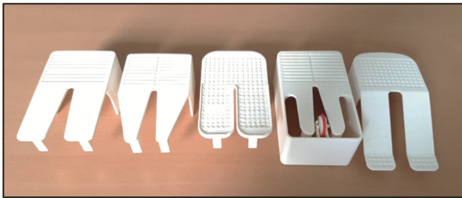
Fig. 2. Prototypes of plug-cases to be used in combination with a regular computer mouse for better accessibility for mouth stick users. From left to right: Versions 1 to 5.
