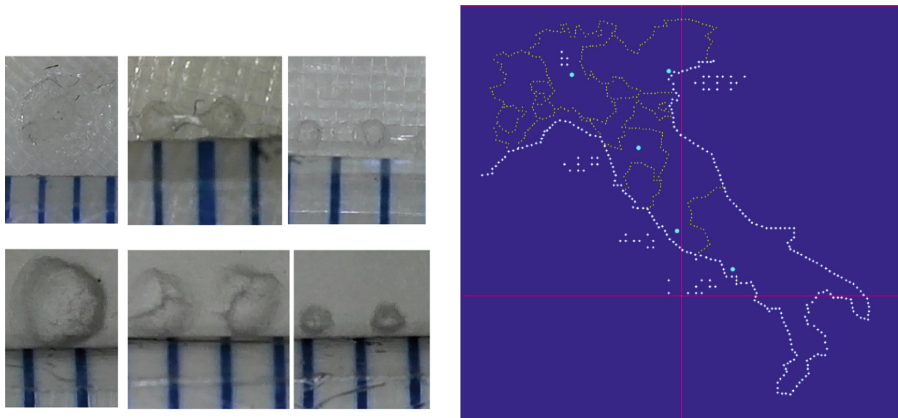
Fig. 1. Three dots embossed by ESA721 (up-left), generated by 3D printer (down-left) and the evaluated embossed dots map (right)
