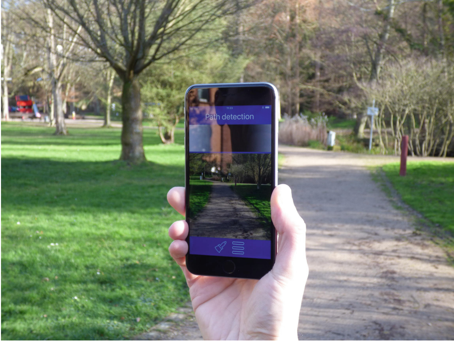
Fig. 4. The detection algorithm was found to be very effective for paths in parks, as well as pavements enclosed by grass. Photo by H. Kucharek.
