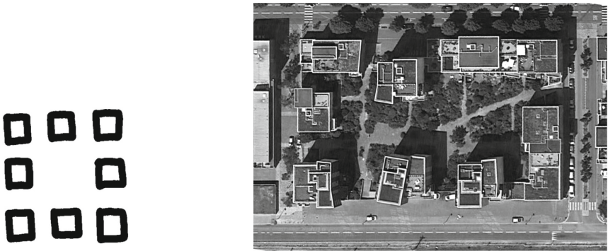
Fig. 4. An open block: diagram (left); example: the urban block designed by Christian de Portzamparc in Nantes, France (right). Image Courtesy of Google Maps.
