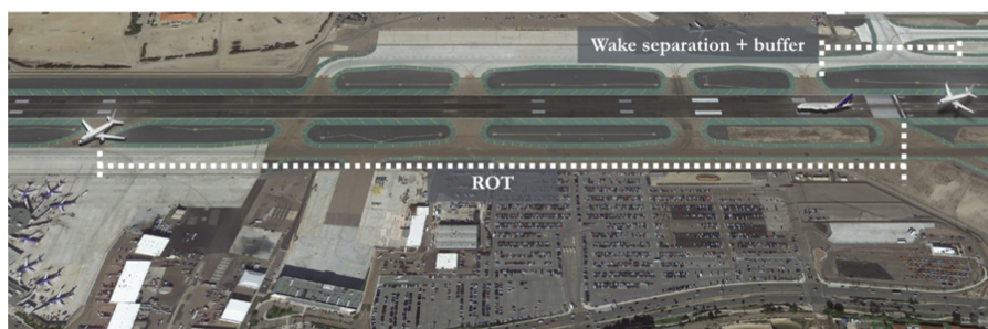
Fig. 2. Wake separation and operational buffer on approach.
