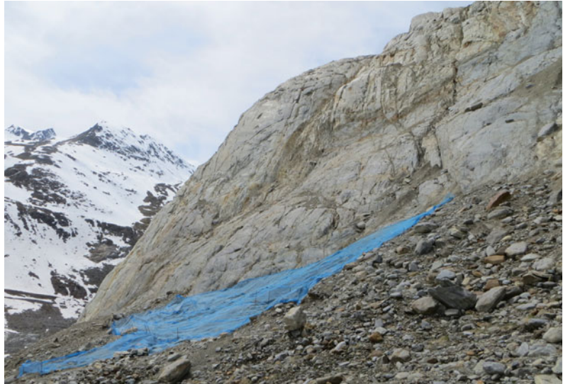
Fig. 9.2 Rockfall collector net in the proglacial zone (2250 m a.s.l.). The contact-line of net and rockwall is 20 m. The lower part of the rockwall is build up by paragneiss, while in the upper part granitic orthogneiss prevails. So, particles from two different rock faces ('rockwall contributing areas') could be accounted with one collector net
