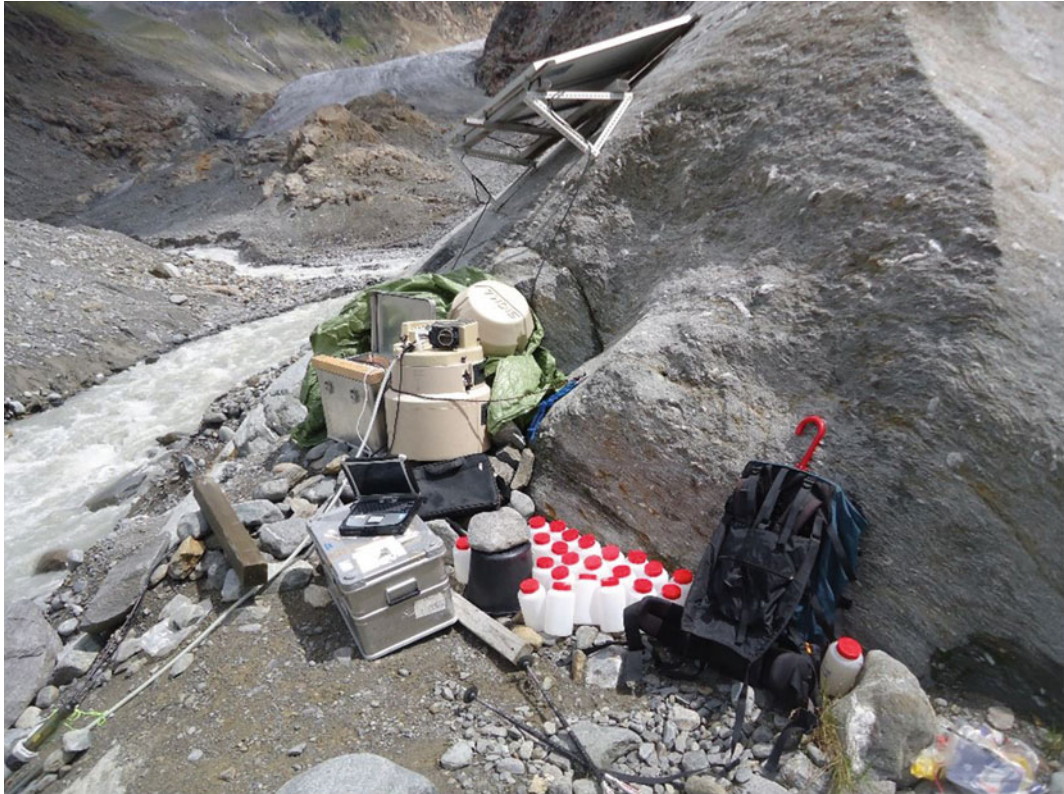
Fig. 13.3 New gauging station installed at the left channel (cs-lc) in 2013, note freshly exposed whalebacks and the glacier tongue in the back (view upvalley, photograph August 18, 2015, David Morche)
