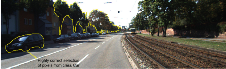
Free-form or polygon selection of objects for labelling in a video frame.
