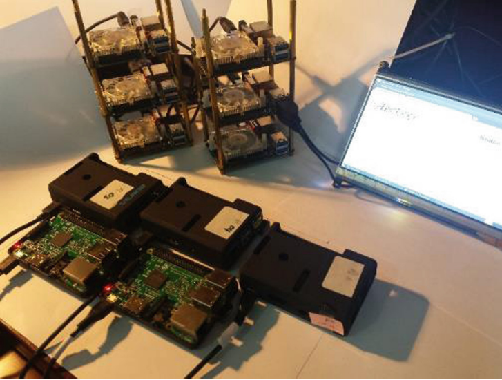
Fig. 1. The LoC4 cluster with 6 Xu4 (Rack mounted) and 5 RPi 3B in cases.
