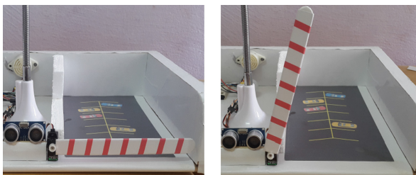
Fig. 21. The opening of the portal when the plate is recognized
