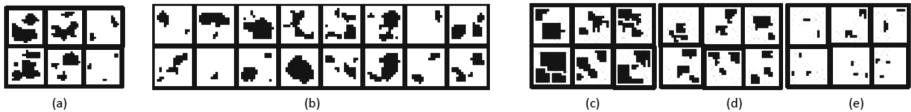
Fig. 1. (a) Examples of images from train sets with two and three grains; (b) Examples of images generated by a GAN on the dataset with two grains. Examples of generated images with (c) d \in [40, 50) , (d) d \in [60, 70) , and (e) d \in [90, 100] .
