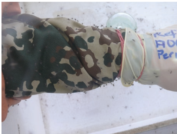
Fig. 12.5 Arm-in-cage test showing excito-repellency including landing, probing and biting behaviour of Aedes aegypti on battle dress uniform fabric treated with 1300 mg permethrin/m 2 prior to laundering
