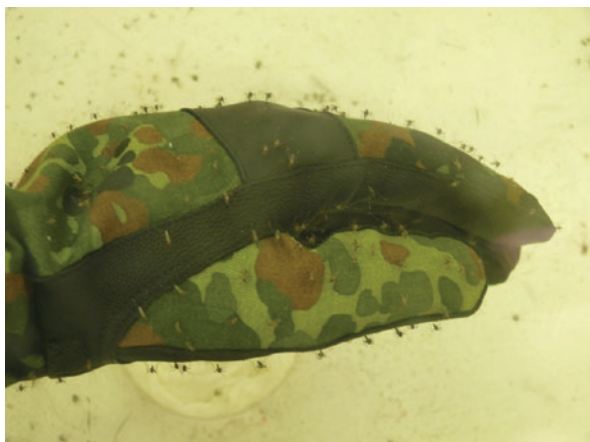
Fig. 12.6 Arm-in-cage test showing landing and probing behaviour of Aedes aegypti on an untreated but bite-proof battle dress uniform fabric. Aedes mosquitoes were not capable to bite through the textile
