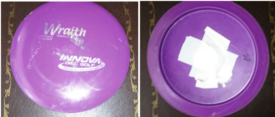
Fig. 3. Innova Disc Golf Wraith Driver disc top view (left) and bottom view with attached Bluetooth tracker (right).
