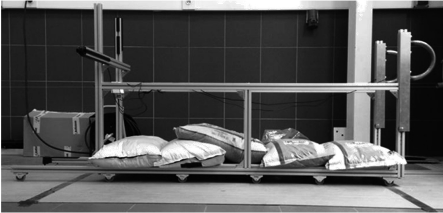
Fig. 1. Dummy bobsled test setup on 12 m wooden track. The sled consists of one push rod for the pilot and two handle bars for the brakeman. Weight and dimensions were adjusted to IBSF rules.
