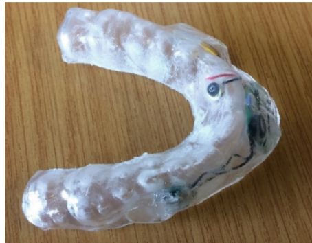
Fig. 1. Prototype of the electronics embedded in the mouthguard.
