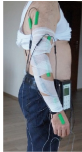
Fig. 2. Sample mounting of goniometers and torsiometer for Subject 2 (Photographs by M. Drzewiecka-Dahlke).
