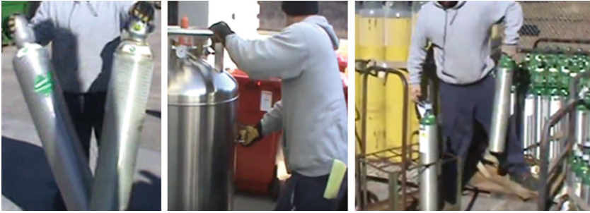
Fig. 1. Left - pulling a dewar; Middle - rolling two cylinders; Right - lifting small cylinders.
