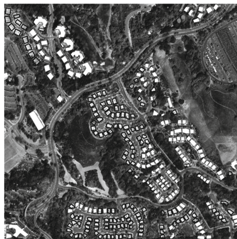
Fig. 8. Small dataset for fine-tuning of the net to the new data. White - unburned buildings, black contours - burned buildings
