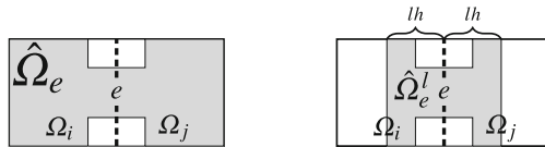
Fig. 1 (Left) Graphical representation of \Omega_e = \Omega_i \cup \Omega_j and \hat{\Omega}_e . The set \hat{\Omega}_e is obtained by removing from \Omega_e all elements which are adjacent to the coarse nodes. From this, we also obtain the interior edge \hat{e} := e \cap \hat{\Omega}_e . (Right) Graphical representation of the slab \hat{\Omega}_e^l corresponding to the edge e
