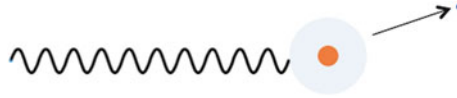
Fig. 5.4 Photoelectric effect. Note that the photon is absorbed by the atom, which expels an electron
