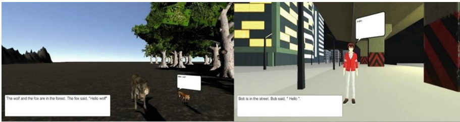
Fig. 2. Output for sentences “The wolf and the fox are in the forest” and “Bob is in the street, Bob said, ‘Hello’”
