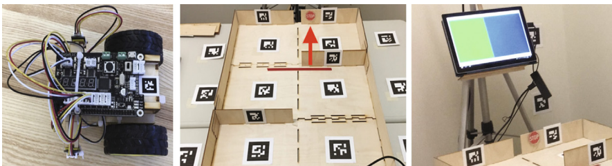
Fig. 1. The material used in the study: the robot that participants had to program (left image), one maze (middle image) and the Kinect-based speech visualization (right side).
