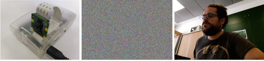
Fig. 3. The IoT camera (on the left), the authenticated encrypted image (in the center), and the original image (on the right).
