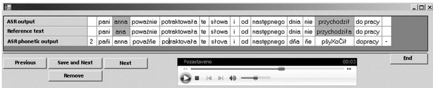
Fig. 1. Program to check transcribed sentences. One can easily compare ASR output, reference text and ASR produced phonetic transcription (incl. silence denoted as ‘-’ and noises indicated by digits). Differences are highlighted. In this example, the first one is due to wrongly typed word ‘ana’ (error in reference), the second was made by the ASR system (omitted ‘a’).
