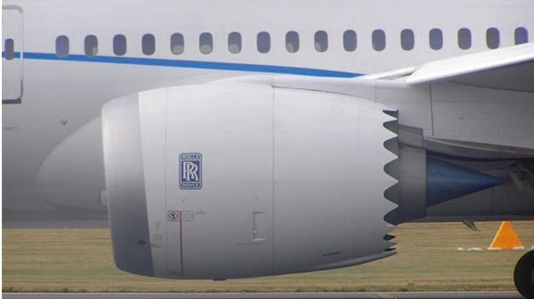
**Fig. 5.36** A photograph of a chevron nozzle in an engine on the Boeing 787 Dreamliner. (source: <https://commons.wikimedia.org/wiki/File:B787-2139.jpg>)
