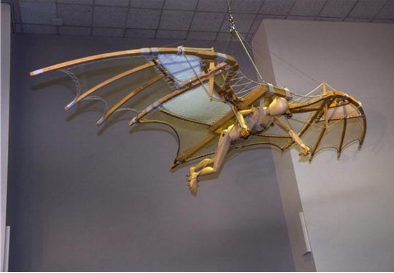
**Fig. 5.1** The ornithopter model at the Smithsonian Institution based on the drawings of Leonardo da Vinci. (Figure used with permission of the Smithsonian National Air and Space Museum (NASM2013-02909. Photo by Mark Avino))
