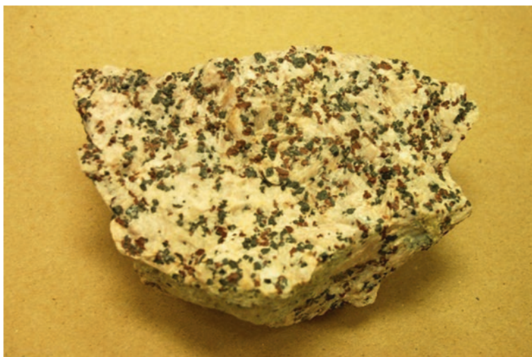
Fig. 3.10 Museum-quality specimen of ore from the Franklin Mine in New Jersey. The ore minerals are franklinite (black) and willemite (red) in a matrix of gangue. (Photograph by B. J. Skinner)
