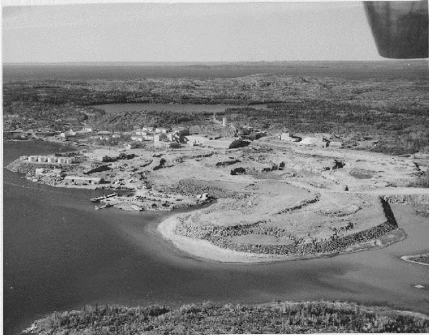
Fig. 3.19 Mine waste and tailings disposal at the Gunnar uranium mine in Saskatchewan
