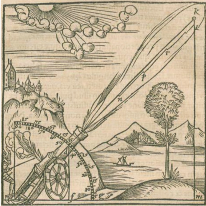
Fig. 2.17 Drawing by Daniel Santbech in 1561 of Aristotle's theory of projectile motion applied to a cannonball. (Santbech 1561)
