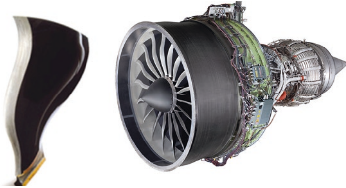
Fig. 5.25 PMC fan blade and casing for engines. ( https://www.geaviation.com/commercial/engines/ge90-engine ; Images used with permission from GE Aviation)
