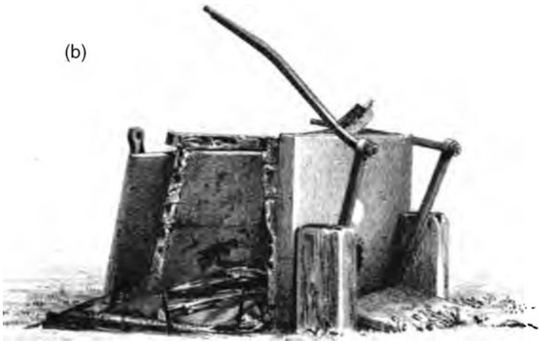
BOX MADE OF 4 INCHES OF IRON, &C., BLOWN TO PIECES BY A STEEL FLAT-HEADED 70-POUNDER WHITWORTH SHELL. RANGE 200 YARDS.
