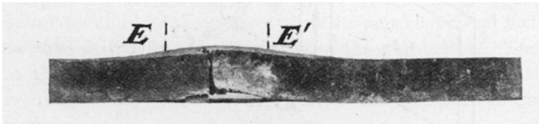
Fig. 2.72 Incipient spall produced in a 1.25-inch-thick mild steel plate by the detonation of a slab of guncotton on the underside. (From Hopkinson 1914)
