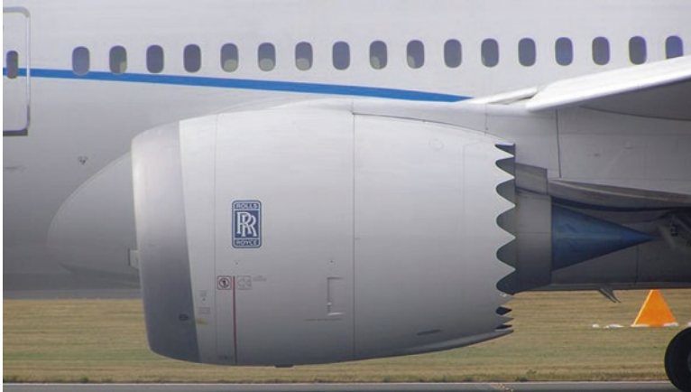
Fig. 5.36 A photograph of a chevron nozzle in an engine on the Boeing 787 Dreamliner. (source: https://commons.wikimedia.org/wiki/File:B787-2139.jpg )
