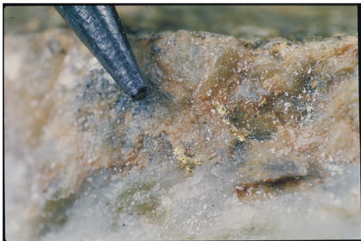
Fig. 3.13 Gold ore from Alaska. (a) Hand specimen. (b) Enlarged view to reveal the gold, seen just beyond the pencil point. Today this is considered to be rich ore. (Photographs by Christopher Barton)
