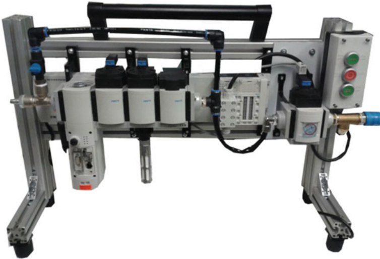
Fig. 9.9 Mobile functional prototype of the smart air-saving unit
