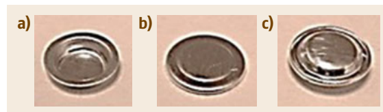
Fig. 24.2a–c Aluminum DSC pans: top (a) and bottom (b) half and assembled pan (c)
