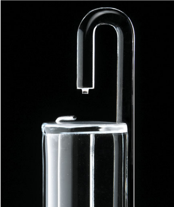
Fig. 24.22 Penetration probe for measuring viscosity behavior by TMA. After [24.41]. Copyright TA Instruments. Used with permission
