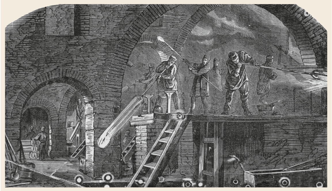
Fig. 1.2 Flat glassmaking by the cylinder method [1.12]
