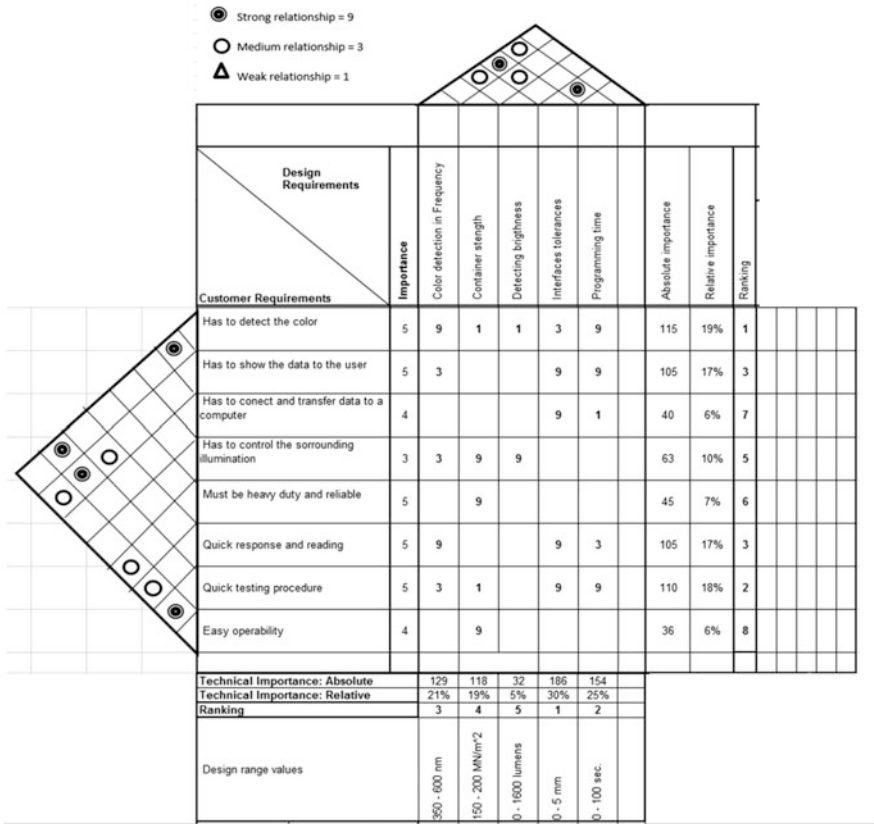
Fig. 6 QFD or the design of the color measuring equipment to determine chassis coloration
