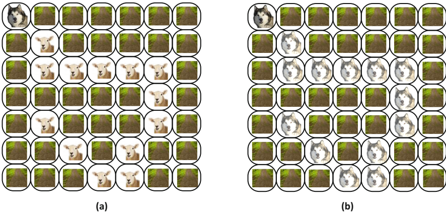
Fig. 3. An example of a wolf movement for the purpose of coding. The wolf starts searching from the upper-left portion of an image and then moves to the first location where he finds a sheep. Then, the wolf finds a sheep in a neighborhood location, thus moves to that location and so on. The relative movement of the wolf can be represented as: LM, SM, SM, SM, RM, SM, CRM, CLM, RM, CRM and SM
