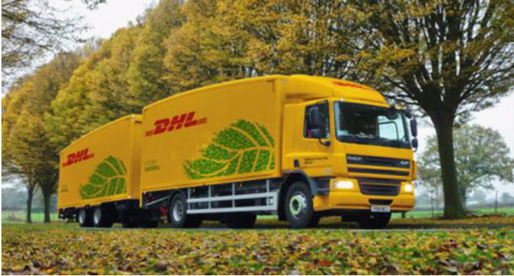
Fig. 7 Teardrop Drawbar Combination
