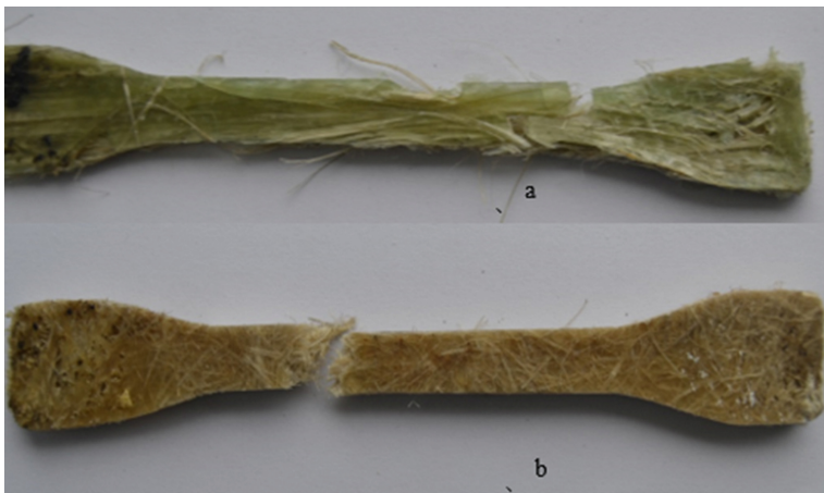
Fig. 5. Samples of composite with fibers I-type (a) and II-type (b) after tensile tests.
