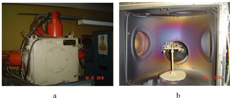
Fig. 2. Installation for applying coatings using the CIB method (a) and a chamber with a device for fixing the specimens (b).
