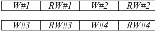
Fig. 2. Intra-instruction redundancy without random number generation, where W : plaintext in word, RW redundant plaintext in word
