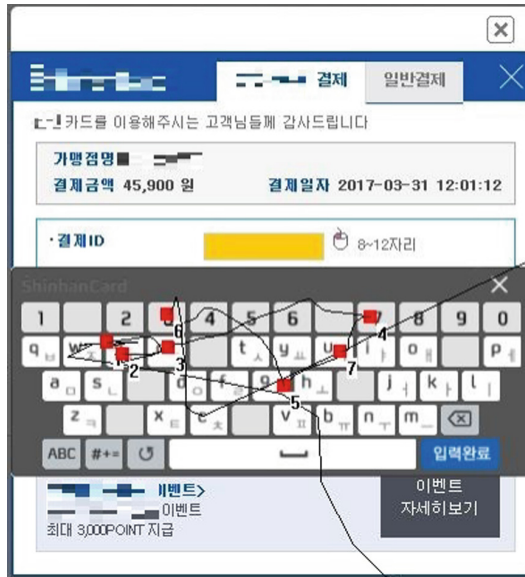
Fig. 3. Stealing mouse data by drawing from the GetCursorPos() function (Color figure online)
