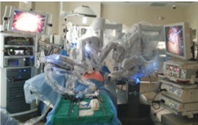
Fig. 28.1 Typical docking of the patient-side cart during robotic foregut and bariatric surgery. The parallel side dock technique allows for ease of access to the head for
