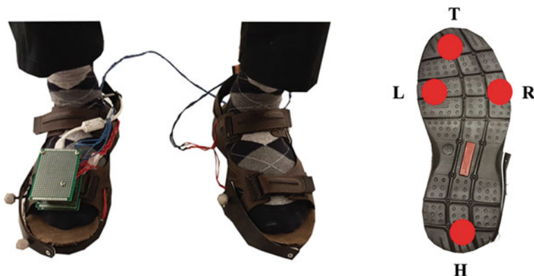
Fig. 16.9 Haptic shoes and positions of foot pressure sensors [23]
