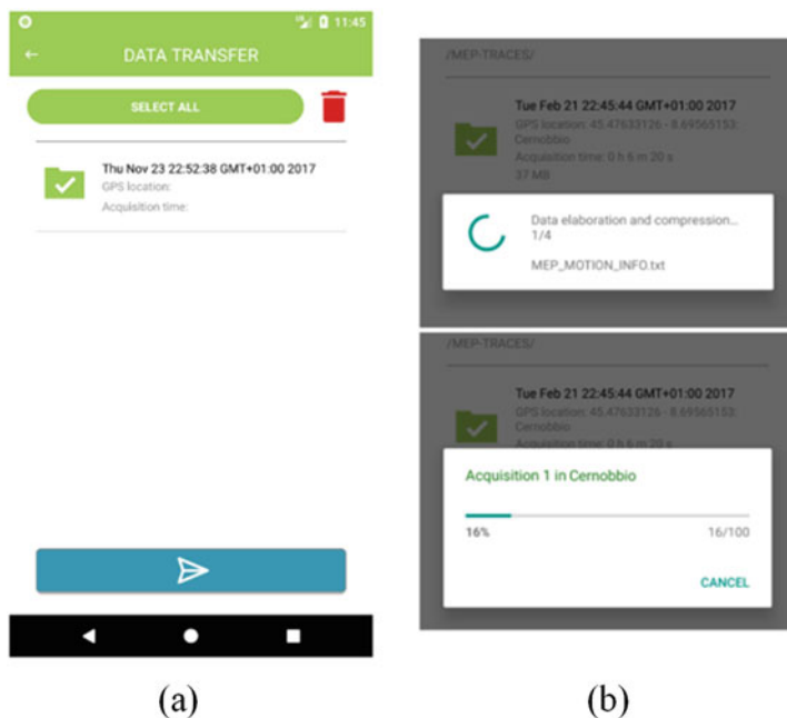
Fig. 6.3 MEP Traces upload interface example: (a) manual selection of all the acquisitions; (b) data compression and connection/uploading task
